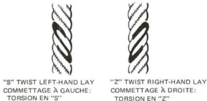
Figure 10-3 The Lay of a Rope Le commettage d'un cordage
