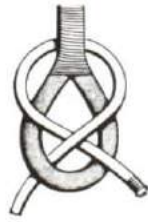
Figure 10-29 Sheet Bend Noeud d'écoute simple
