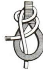
Figure 10-30 Double Sheet Bend Noeud d'écoute double
