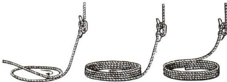
Figure 10-14 To Coil a Rope for Running Lovage d'un courant
