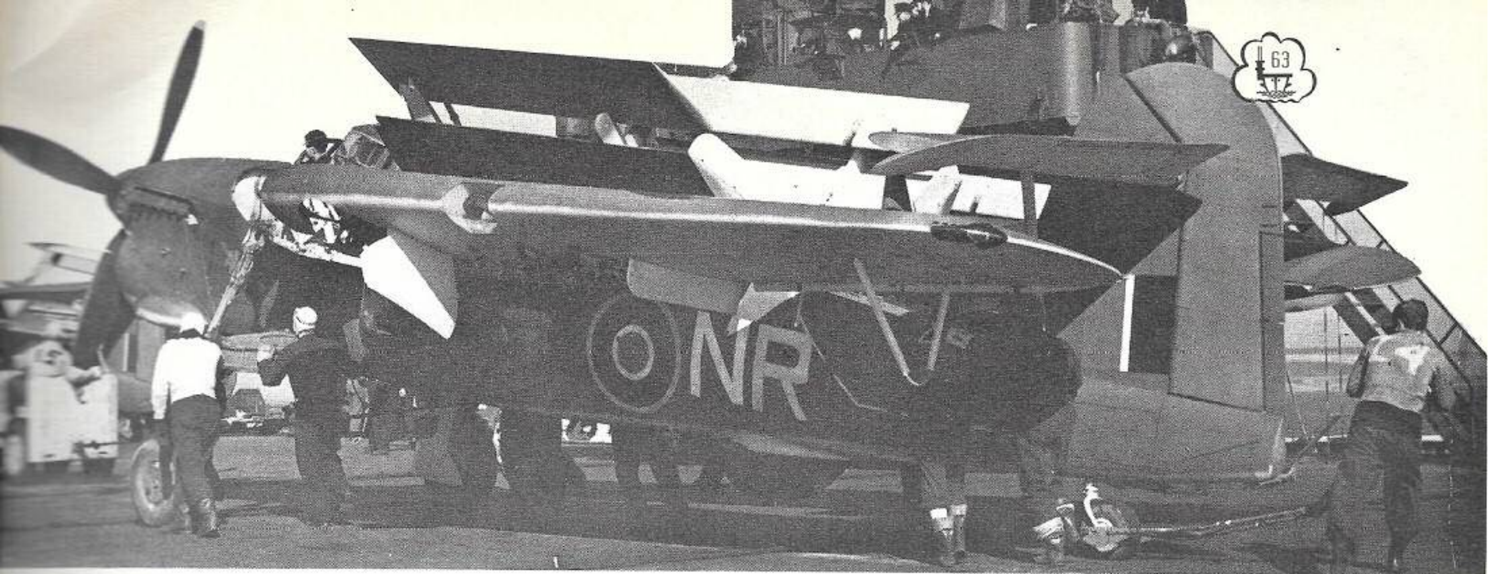
With all planes landed, wings folded, the deck handling party wheels the aircraft toward the forward elevator which takes planes below to the Hangar Deck. Commander D. C. Wallace, D.S.C., R.C.N.R., and Lt.-Cmdr. (F) Paul G. Godfrey, R.N., look down from the bridge.
