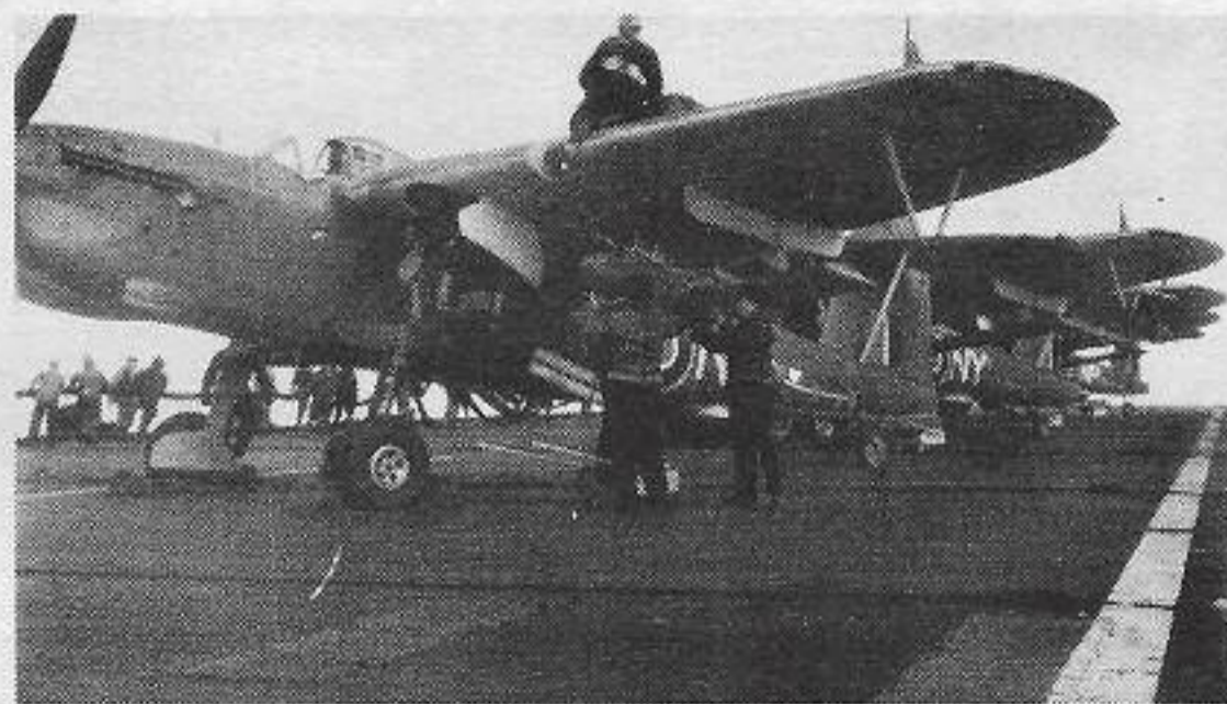
The planes equipped with rockets are loaded with a bomb load for test of lifting capacity
