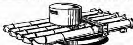
QUINTUPLED 21-INCH TORPEDO TUBES WITH ARMoured CUPOLA AS FITTED IN WORLD WAR II BRITISH DESTROYERS.
