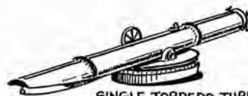
SINGLE TORPEDO TUBE (EARLY TORPEDO BOATS)
