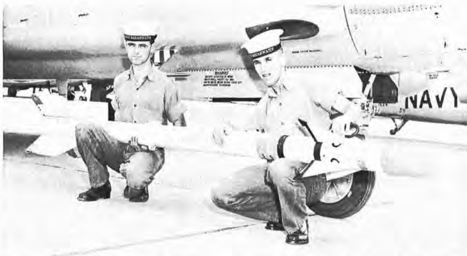
The Sidewinder guided air-to-air missile is carried by RCN Banshee jet fighter aircraft. (DNS-21041)
