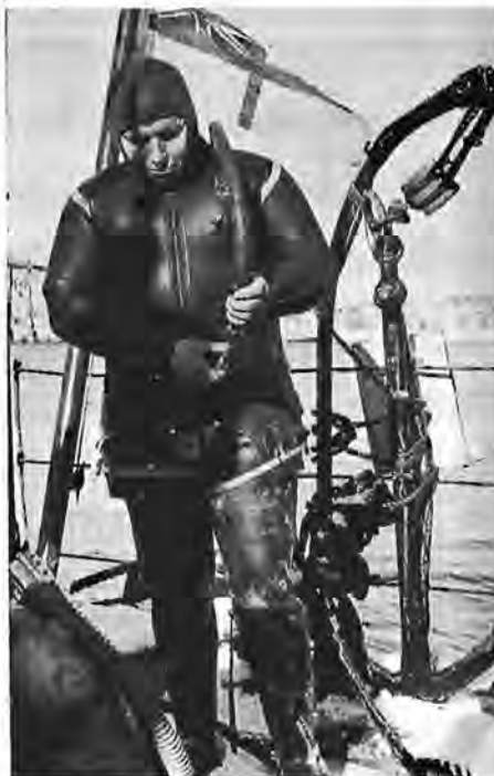
Ldg. Sea. Lloyd (Chuck) Doyle, of HMCS Granby , clearance diving depot ship in Halifax, flushes hot water through a new type of diving suit, designed by a West Coast diver, Ldg. Sea. W. H. Nehring, to keep divers warm in chilly winter waters. (HS-74203)
