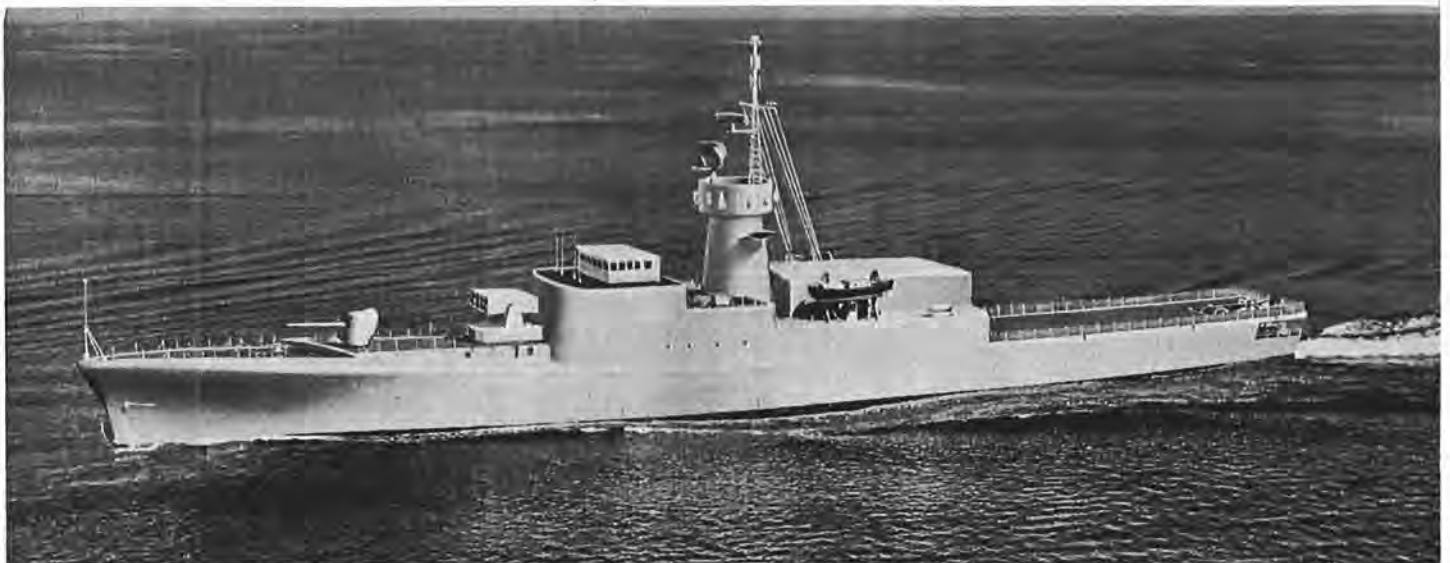
Four helicopter-equipped destroyers (DDH) will be built under the five-year equipment program announced on Dec. 22. The new ships will be slightly larger than the Annapolis class destroyer escorts, will have the latest anti-submarine detection equipment and will carry CHSS2 Sea King anti-submarine helicopters. They will have a five-inch gun for shore bombardment and surface action, and provision will be made for later installation of a missile defence system. (CN-6857)
