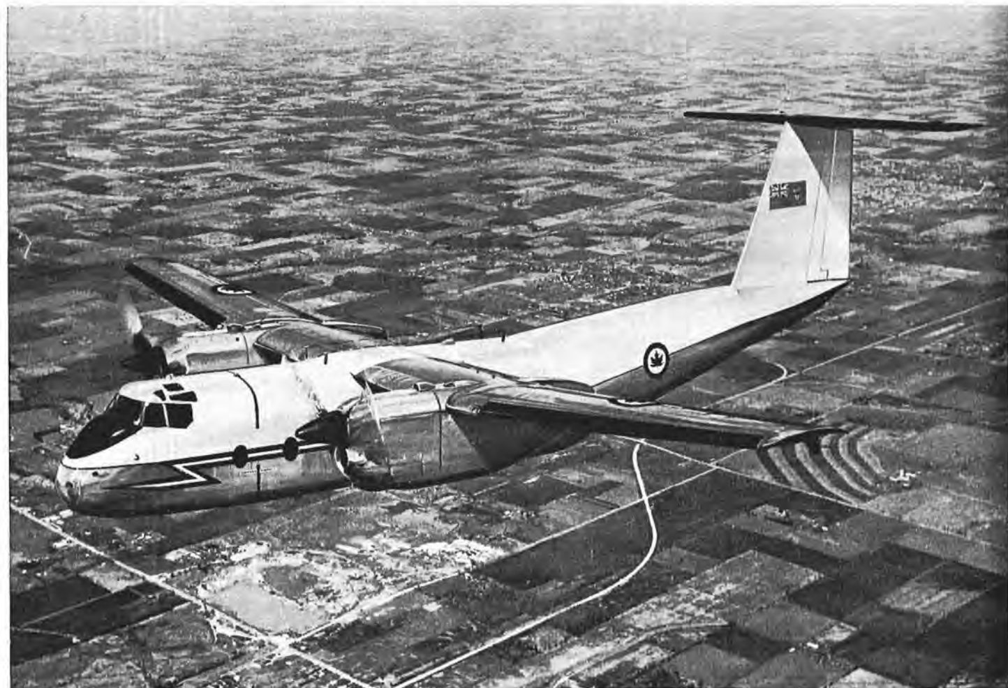
The Buffalo aircraft to be supplied to the RCAF is a medium transport, built by the de Havilland Aircraft of Canada. It can airlift 41 fully equipped soldiers or 35 paratroops over 700 miles and return to base when long-range fuel tanks are installed. As a cargo carrier, it has a five-ton-plus capacity and is designed for short take-offs on rough ground. (PL-145048)
