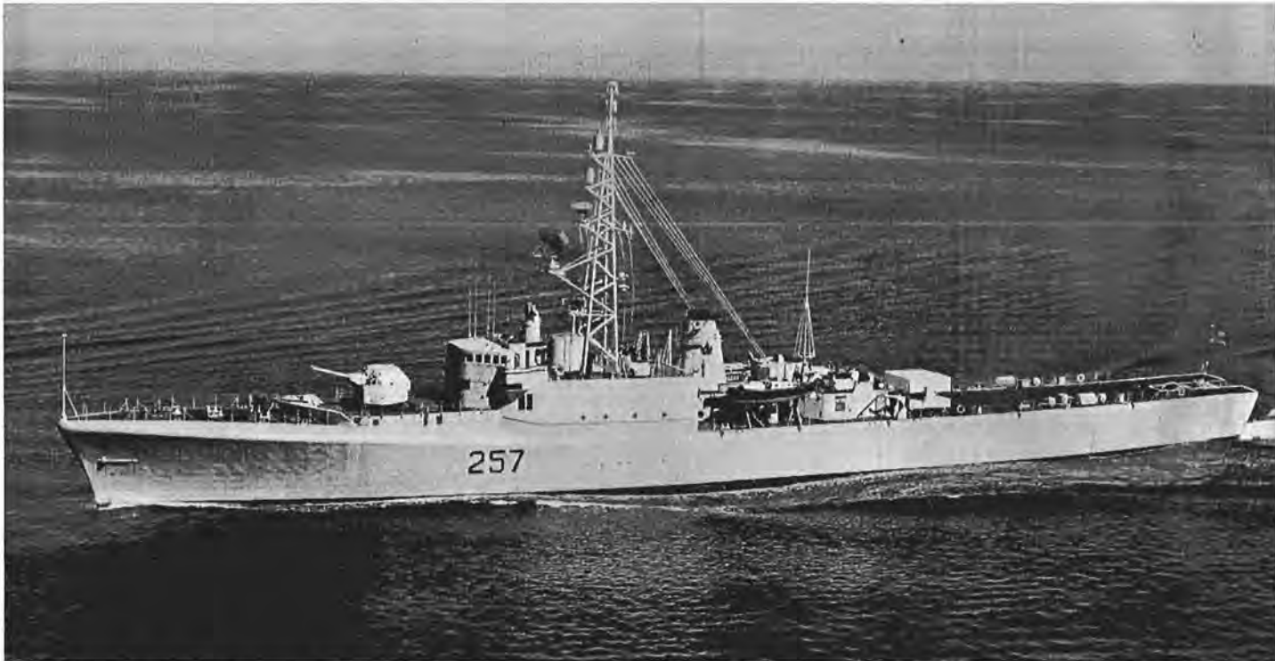
This year will see the beginning of the progressive conversion of seven Restigouche class ships with a view to increasing their ability to detect and attack submarines. Variable depth sonar and other equipment designed to improve detection capabilities will be installed and the ships will be equipped with a rocket-assisted homing torpedo delivery system (Asroc). (CN-6852)
