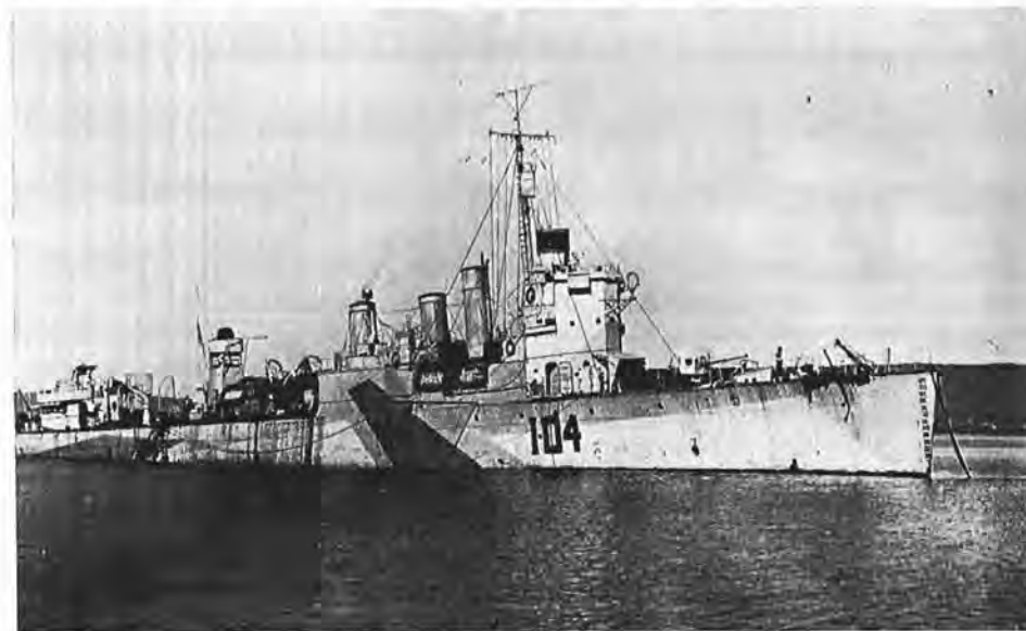
One of the old U.S. destroyers given to Britain in the Churchill-Roosevelt destroyers-for-bases exchange, the Annapolis was transferred to the RCN as a four-stacker, but later had one stack and boiler removed to improve her sea-keeping qualities. It was in the latter form she was known to thousands of Canadian sailors at Cornwallis, where she was a training ship. (A-31A; DB-0430-AT)
