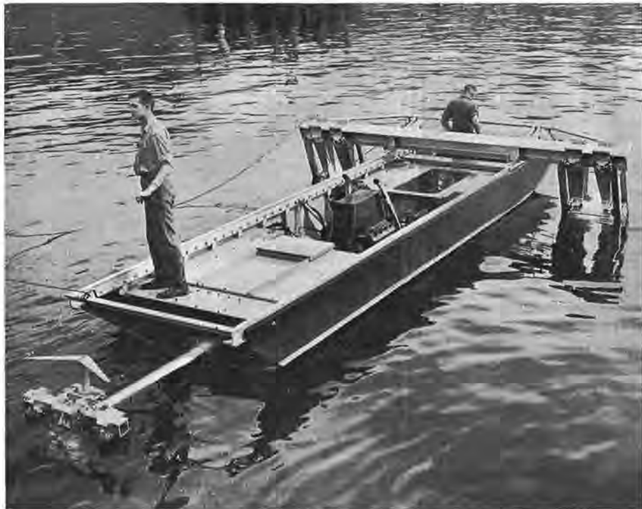
This strange craft, called the “R-X”, will be used this spring to test a set of super-cavitating hydrofoils in the continuing search for the most effective design for high-speed hydrofoil boats. Super-cavitation involves the deliberate formation of an air or vapour cushion on the blade of a foil or propeller. All is made clear in the article accompanying this picture. (Naval Research Establishment, Halifax.)
