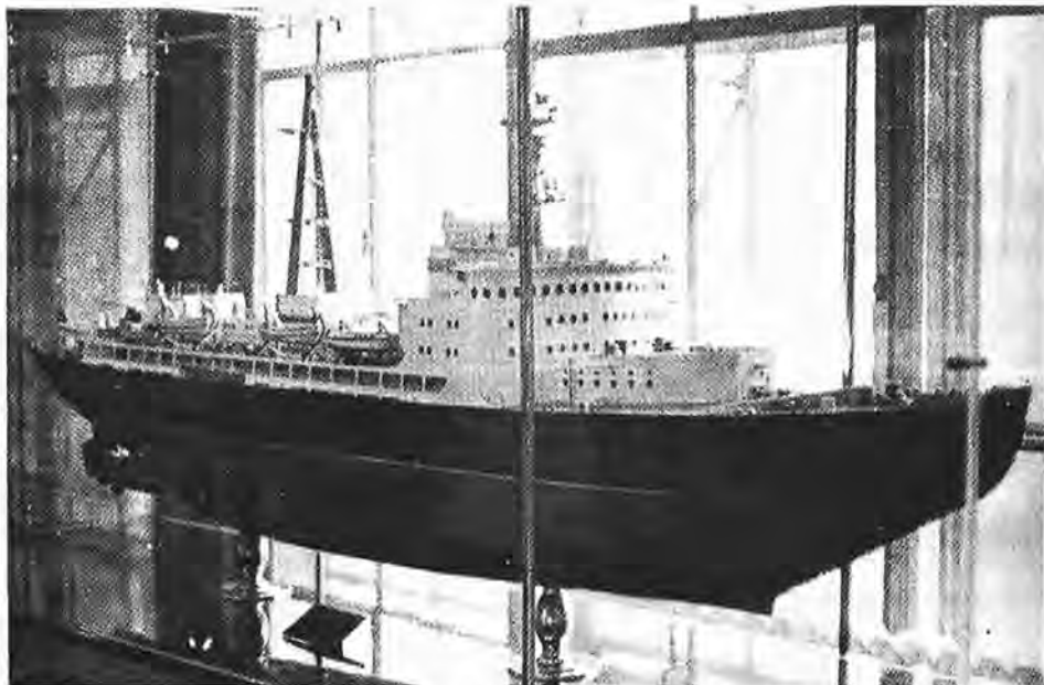
Here are two views of a model of the Russian nuclear-powered icebreaker, Lenin , launched late in 1957. Her engines will develop from 44,000 to 56,000 horsepower and she will have three propellers, giving her a maximum speed of 18 knots. It is reported that the Lenin will be able to steam for a full year without refuelling and that her daily fuel consumption will be five ounces.
