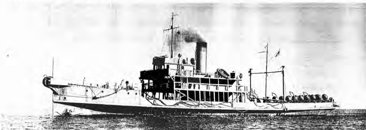
Remember the Sankaty? She carried out a number of assorted duties during the Second World War around Halifax and is shown here putting out for the harbour approaches with a deckload of controlled mines—the kind that are fired from a shore control point when the presence of an enemy ship or submarine is known or suspected. (H-142)
