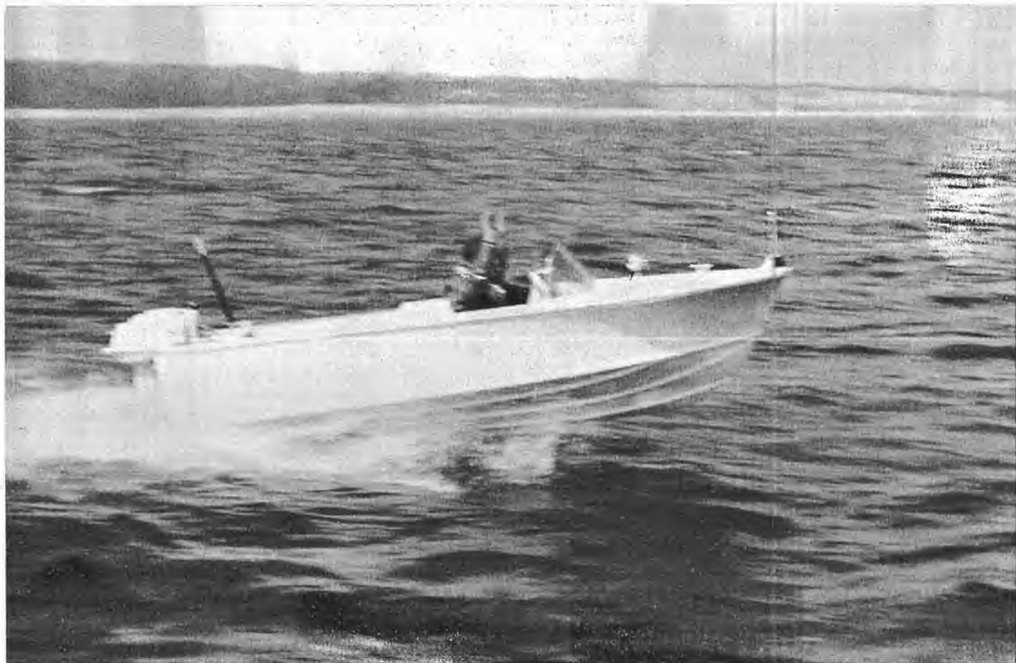
"Look, Mal No hands!" The Hunt 14-foot hydrolift hull is shown under test for the maintenance of longitudinal stability. (O-13816)
