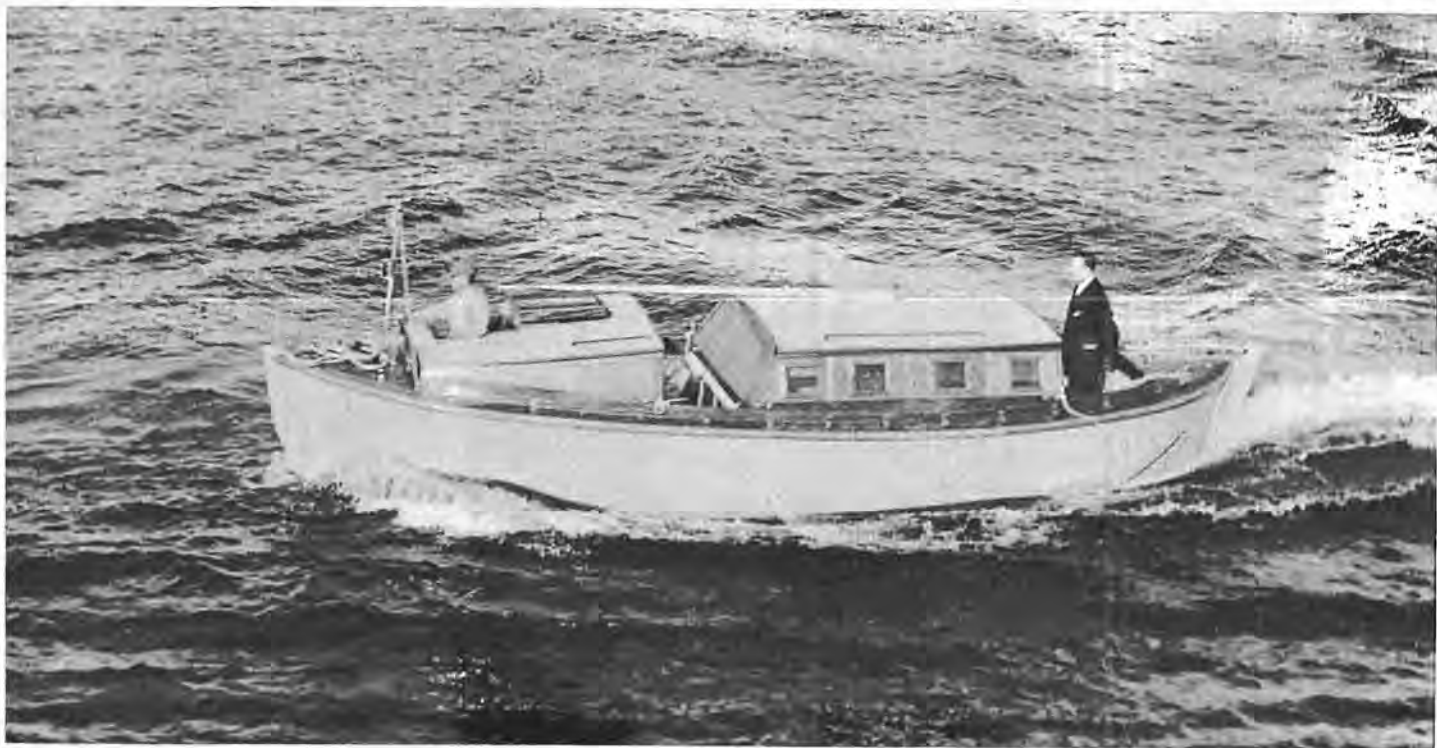
Traditional wooden construction, double-ended motor seaboat; weight, 6,000 pounds; length overall, 27 feet; beam, eight feet; passenger load, 25; stores capacity, one ton. The writer calls it "ponderous and inefficient". (O-6033)
