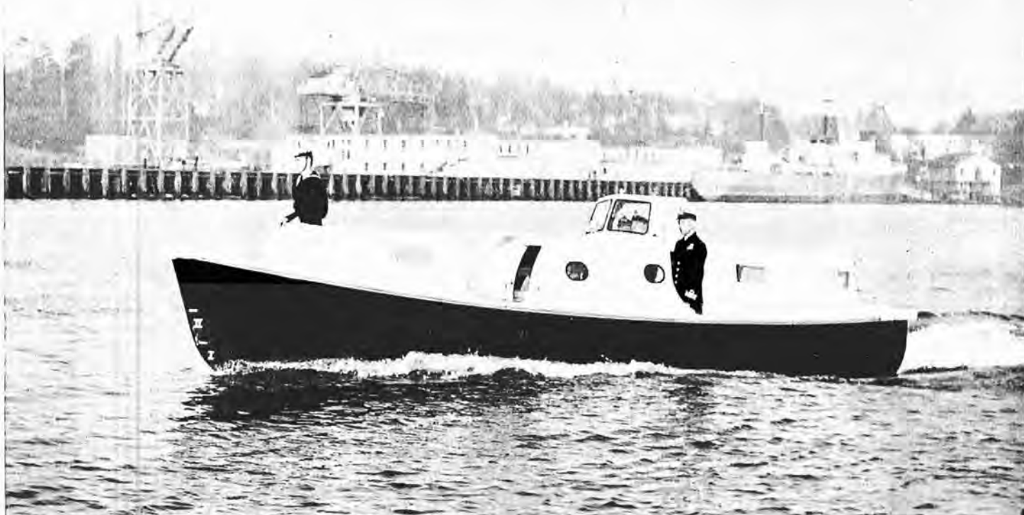
Newly designed all-fibreglass construction motor workboat; weight, 5,000 pounds; length overall, 27 feet; beam, eight feet; passenger load 30; stores capacity, two tons. (E-63724)
