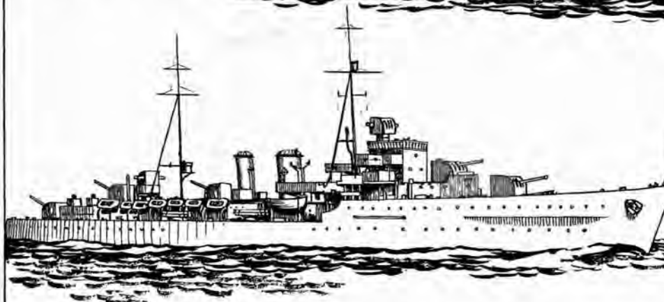
H.M.S. DIOMEDE (RIGHT) DIFFERED FROM HER SISTERS IN THAT HER FORWARD GUN WAS MOUNTED IN A GUN-HOUSE AND THERE WAS NO BLAST SCREEN ON THE SHELTER DECK. NOTE AIRCRAFT PLATFORM ABAFT FUNNELS.
