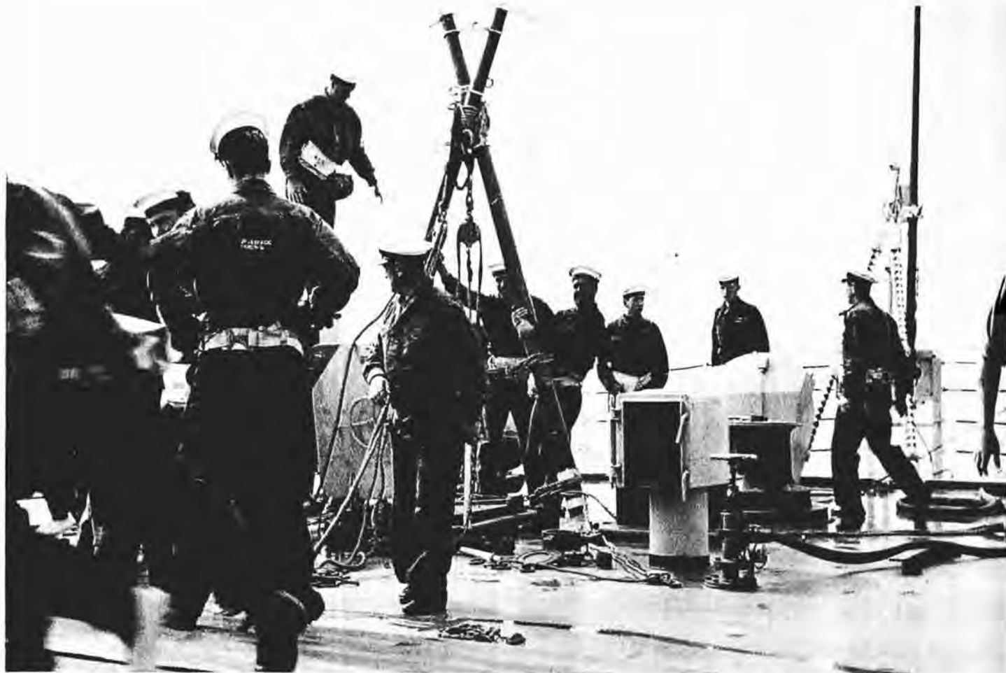
Rigging sheerlegs is a favourite test of seamanship during General Drill and, considering the shortage of spare spars in modern warships, some ingenuity is required. This and other pictures illustrating the accompanying article were taken on board the 'Gatineau during last year's Portugal cruise. Ships in company were the Terra Nova, St. Croix and Kootenay. (O-13123-36)
